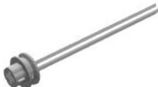
Step 2: Add a 20X30 medium balloon wheel to the axle, touching the offset pulley.
