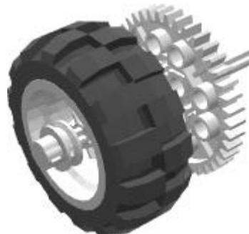
Step 6: Take a 10 stud axle and add an offset pulley to its end.
