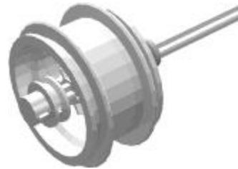
Step 4: Add a 40 tooth gear to the axle, touching the rightmost bush that is already on the axle.
