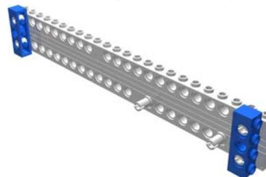
Step 7: Attach a 1X8 beam to the side using the remaining two black pegs
