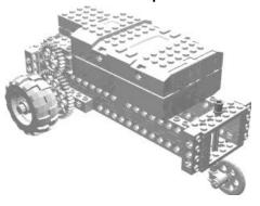
Step 3: Attach the electric plate of a short electrical cable to Output Port A on the RCX. Attach the plate at the other end of the cable to the left motor of the robot.
