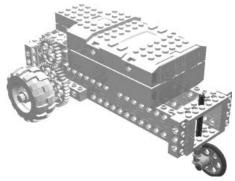
Step 2: Attach a bush to the end of the vertical axle that is sticking through the top plate. Make sure that it is not on so tight that the vertical axle cannot freely rotate in the two plates.
