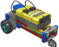
Step 1: Take the complete chassis that was constructed in Stage 6. Take the wheel assembly that was constructed in Stage 7. Pass the long, vertical axle of the wheel assembly through the middle hole of both of the 2X6 plates that are at the front of the chassis.
