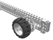
Step 7: Attach another offset pulley to keep the wheel in place on the axle.
