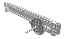
Step 4: Place two bushes on the axle, adjacent to one another, and against the gear. They will hold the gear in place.
