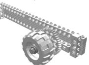
At this point, the left side of the robot chassis is now complete. The next stage is to build a mirror image of this assembly that will serve as the right side of the robot chassis.
