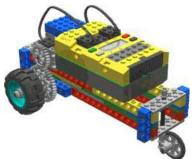
Step 2: Take the light sensor assembly that was constructed in Stage 9. Press it down to connect it to the front of the robot chassis, using the free studs in front of the RCX. Then connect one of the light sensors to Input Port 1 on the RCX, and the other light sensor to Input Port 3.
