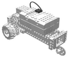
Step 4: Use another short electric cable to connect RCX Output Port C to the motor on the robot's right. The orientation of this connection will have to be adjusted to ensure that the two motors spin the wheels in the same direction. Conversely, the direction that the motors spin will have to be set in the software that runs the robot.
