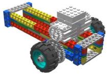
Step 4: Attach the RCX brick directly to the chassis directly in front of the two motors. There should be two free studs on the sides of the robot in front of the RCX brick.
